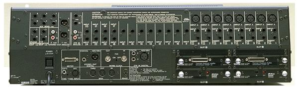
Monitoring to amplifier and speakers is from the Control Room or Studio Outs (1/4" TRS) connections Program Out is from the STEREO OUT ANALOG (XLR) connections
