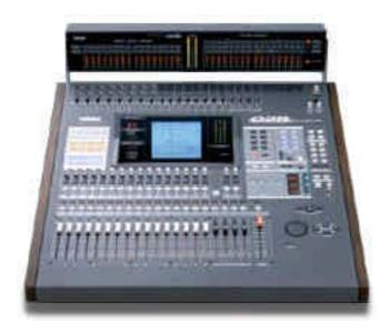
The Fastrack VS hybrid editing system interfaces to the Yamaha 02R Digital Audio Mixer with a 6-pin DIN to 9-pin RS-422 serial control cable and Yamaha 02R audio mixer MIDI protocol. Direct control of each individual fader and the learning of manual adjustments are possible.
